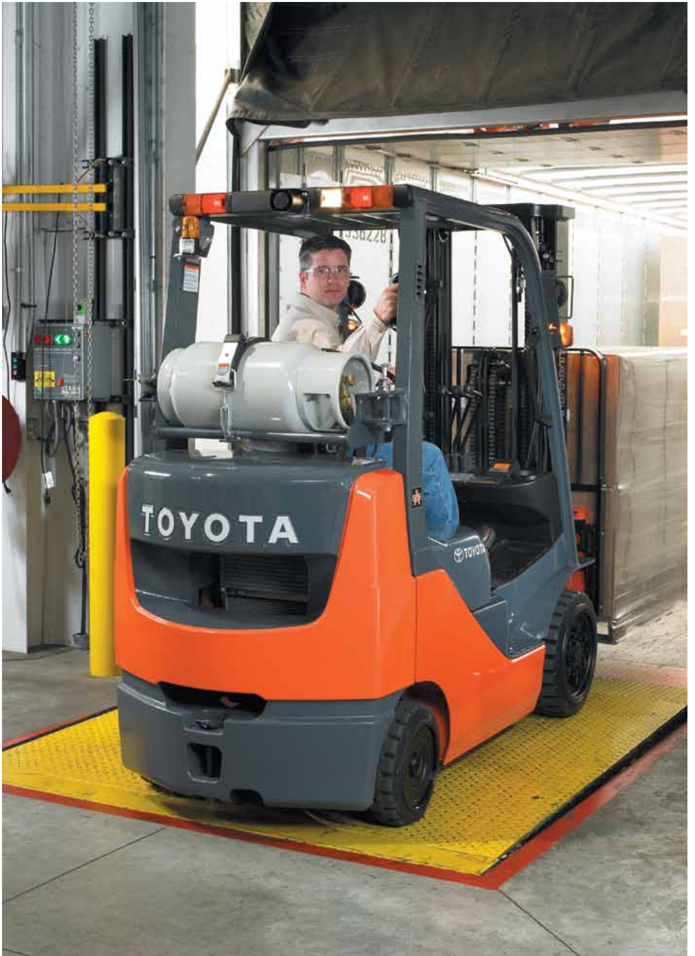
Cushion tyre technology allows easier handling of heavy loads in restricted spaces.
